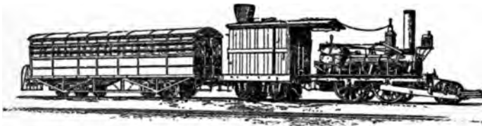
Cars and locomotive in use on the Camden & Amboy Railroad in 1845. The cars were heated by wood stoves, the glass sash was stationary, and ventilation was possible only from a wooden-paneled window which could be raised a few inches.
